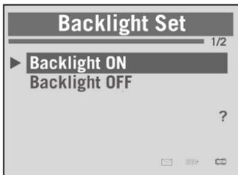
3) Press the **Y** button to confirm change or press the **N** button to exit without change.
