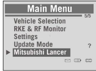
1) Use the **UP** or **DOWN** Arrow button to select the vehicle from the Main Menu, place the tool alongside the valve stem of each wheel and select the **Y** button.
