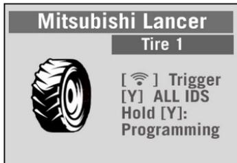
4) A screen will display the correct sensor (frequency type) to program for the selected vehicle and the sensor ID to be programmed.
