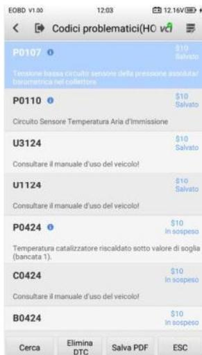
Figura 7-16 Schermo DTC e FFD
