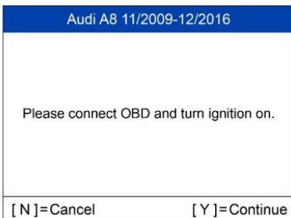
Follow the onscreen instructions to connect the tool with the test vehicle via OBDII cable. Turn on the ignition. Press **Y** to continue, and the tool will automatically read the sensor IDs and Data Trouble Codes (DTCs) present in the ECU.
