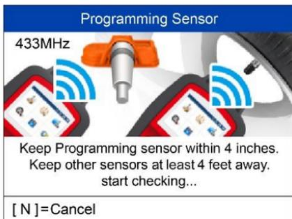
Place a new MX-Sensor in the sensor slot or hold the top of the tool close to the sensor to program.
