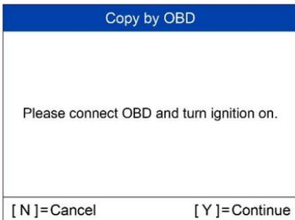
Follow the onscreen instructions to connect the tool with the test vehicle via the OBDII cable. Press **Y** to continue, or press **N** to exit.
