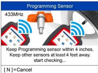
Place a new MX-Sensor near the top of the tool to program.
