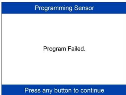
A failure message will display if the sensor fails to program. Press any button to continue. Ensure you are using an MX-Sensor are that you are using the correct frequency. Try to program sensor again.
