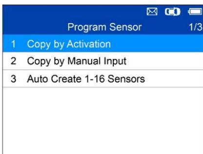
Press **Y** to select Copy by Activation. Place the tool near the sensor to be copied. If the sensor is still attached to the wheel, hold the close to the tire sidewall right above the sensor.
