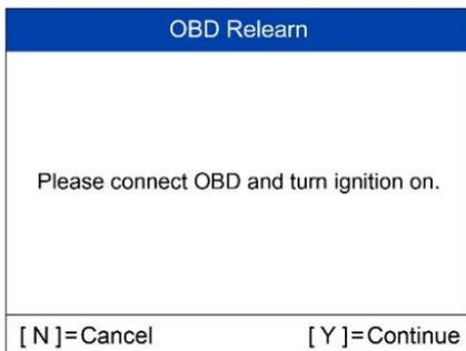
Follow the onscreen instructions to connect the tool and vehicle via OBD cable and turn the ignition on. Press **Y** to continue.
