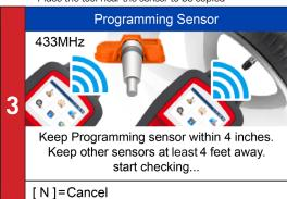
• Place a new MX-Sensor near the top of the device to program
