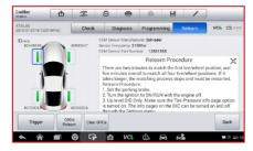
ALL SYSTEM DIAGNOSTIC Sensor position relearn assist procedure
